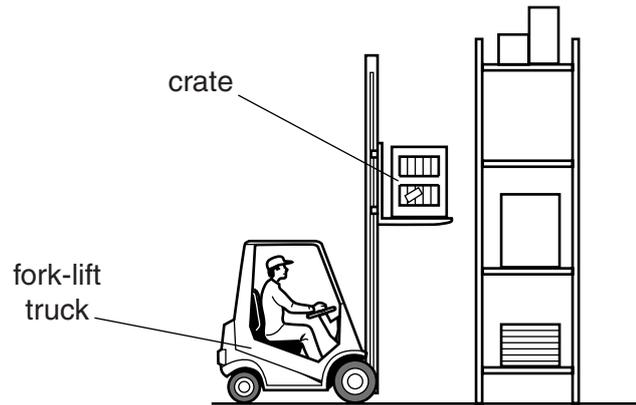
The fork-lift truck lifts a crate of weight 640N through a vertical distance of 3.5m in 4.0s.
