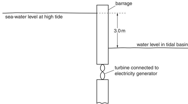
At high tide,  $1.0\text{m}^3$  of sea-water of density  $1030\text{kg/m}^3$  flows through the turbine every second.
